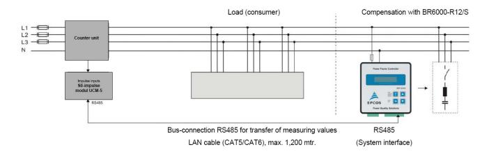
Set-up of a measuring system for recording of different counter values (e.g. for cost centre management). Up to 32 devices can be operated at the bus (MODBUS –RTU), even mixed with other devices as for example MMI6000 or MMI7000. Display and evaluation of measured values is done on PC with the software "MMI-energy" that is included in the delivery.
